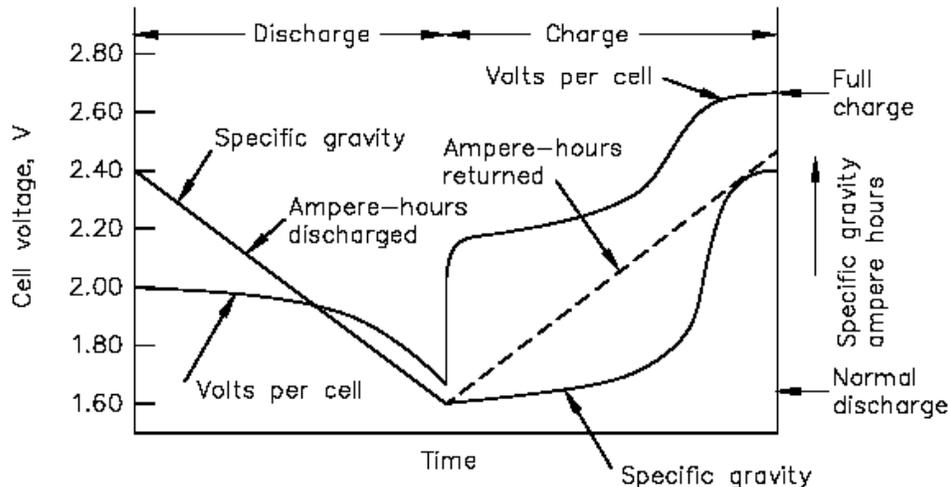
OCV Plots on the downward sloping line for the specific gravity during discharge can be estimated by using the following equations:
